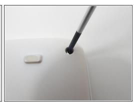
Remove four 5 mm Phillips #00 screws from each corner of the tablet.
