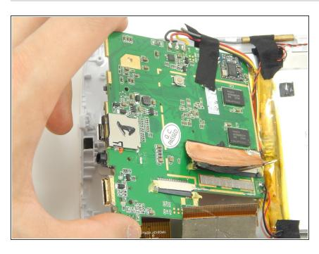
Gently lift up the motherboard and reorient it in a more efficient manner in order to locate the desired components.
