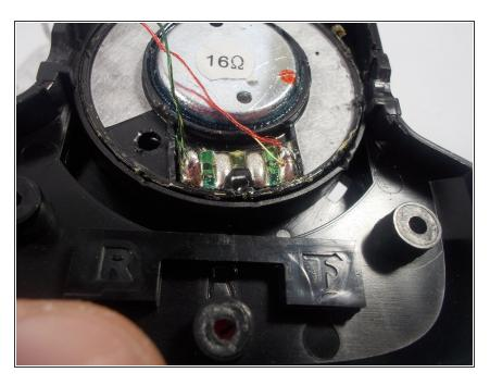
Solder the wires you disconnected from the old speaker to the new speaker. The red wire is to be
