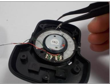
Insert your new speaker into the circular shaped slot located on the speaker cover.
