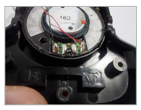
Disconnect the red and green wires from the 16 Ohm speaker.
