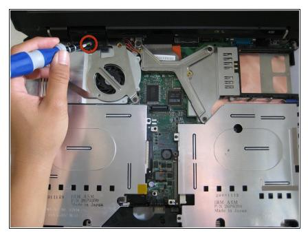
Remove the 5.6mm screw that holds the LCD to the upper case.
