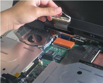
• Pull out the white tab connecting the LCD to the motherboard.
