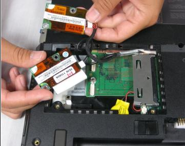
• Remove the four 9.1mm screws attached to the modem and ethernet cards.
