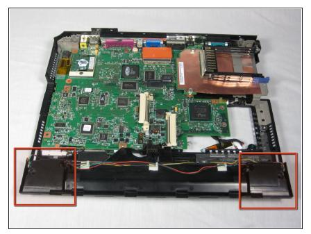
Locate the speakers on the bottom left and right of the ThinkPad A30.
