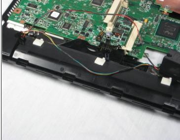
Remove the wires from the white tabs by lifting the black wire casing.
