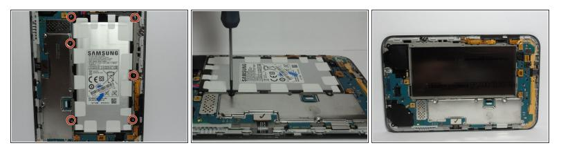
Using the Phillips precision screw driver remove the six 4 mm screws holding the battery in place.
