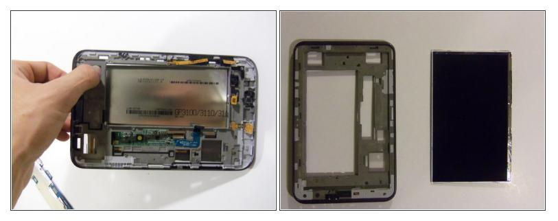
• Press gently from the back of the device to loosen the LCD screen until it separates.
