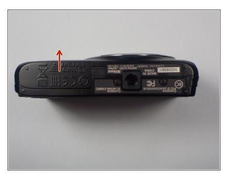
Open the battery cover by lightly pushing on the cover and sliding it forward
