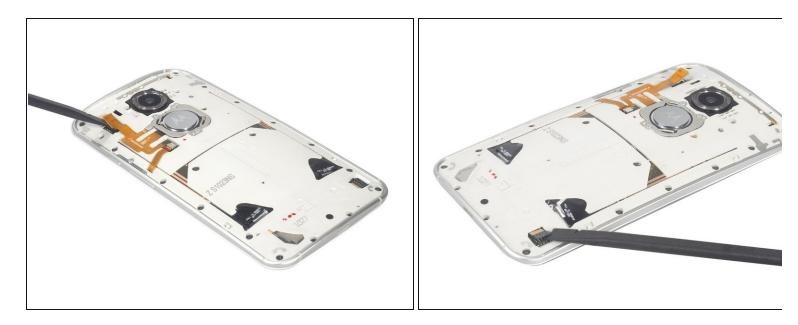
• Release power button connecting flex connector and battery connector.
