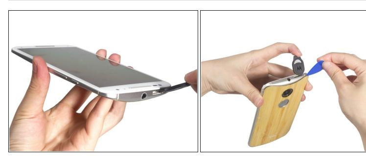
Push the eject pin to open a gap and place a guitar pick into the gap.
