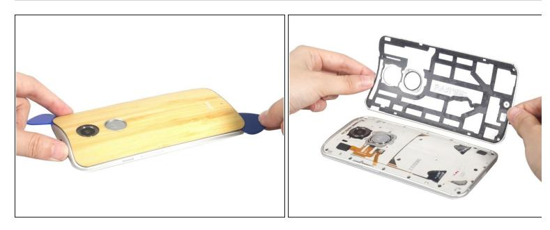
Slide the guitar pick to cut the adhesive sticker and peel off the soft back cover carefully.
