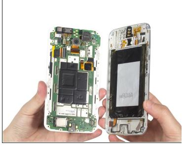
Twist off all 18 black torx screws and remove middle housing from front assembly.
