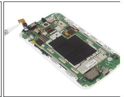
• Release front camera connector and remove it.
