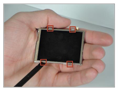
• Pry the LCD display out from the four metal clamps.
