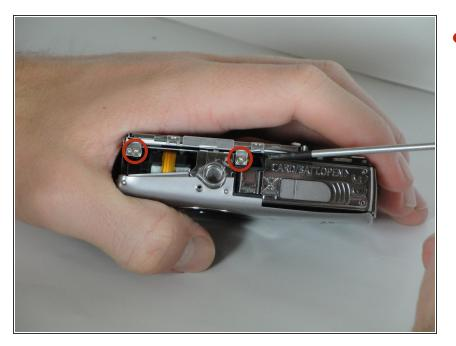
Remove 2 2.4mm screws on bottom.
