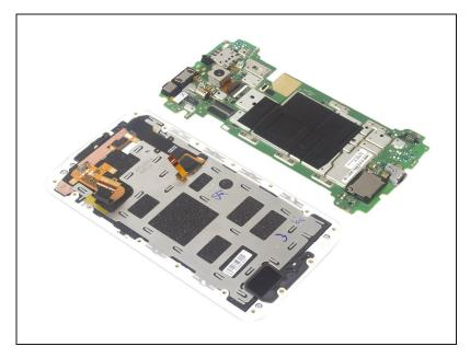
• Tips: The LCD screen is difficult to separate from bezel even though by heat. So you'd better prepare the screen replacement parts with bezel together. And the metal shield can be removed easily.
