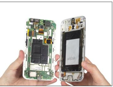
• Twist off all 18 black torx screws and remove the front assembly from middle housing.
