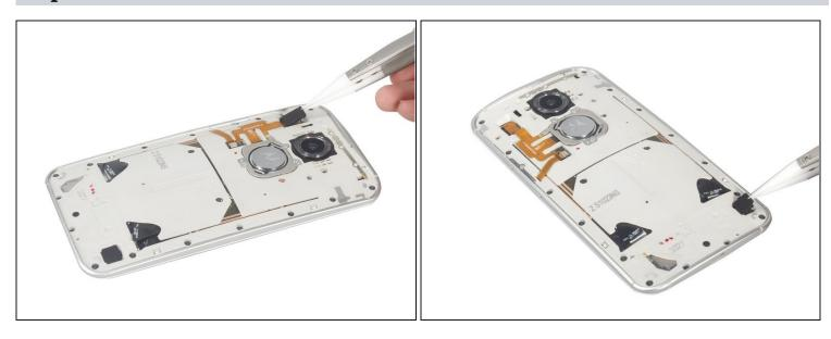
• Remove those two rubber covers which securing power button connecting flex connector and battery connector.
