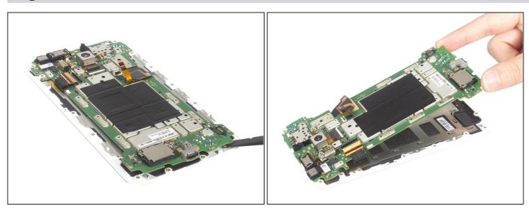
• Pry up the motherboard from right and bottom corner. Remove the LCD screen from motherboard.
