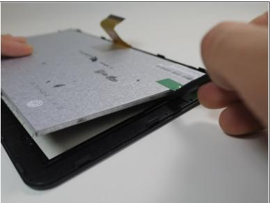
After removing the motherboard, use the black nylon spudger to pop the screen out of the housing holding it to the front of the screen case.
