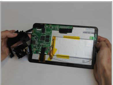
Begin removing the black tape covering the motherboard inside the tablet.
