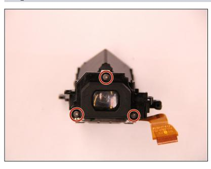
Remove the viewfinder assembly from the camera. The screws that hold the eyepiece in place are accessible. Remove these 3 screws from the rear face of the eyepiece. Two screws are located at the bottom and one screw is located on top.
