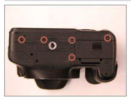
Remove the 7 screws from the bottom of the camera using a Phillips screwdriver
