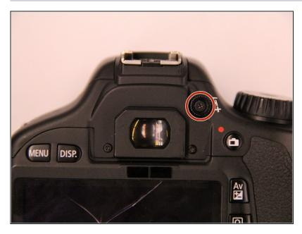
Remove the screw in the center of the viewfinder focus knob located to the right of the eyepiece.
