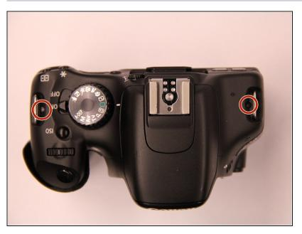
On the top cover, remove the two screws from under the metal tabs that are used to attach the camera straps.
