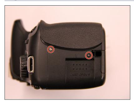
• Remove the two screws on the right side of the camera.
