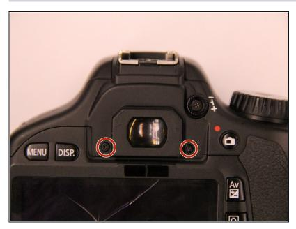
Remove the two screws beneath the eyepiece
