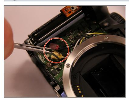
On the lower left side on the front of the camera, disconnect the red and yellow wires from the circuit board.
