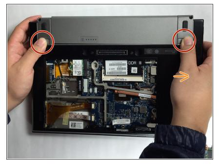
Push each slide towards the edge of the device. This will cause the battery to release.
