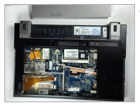
Remove the battery from the device.
