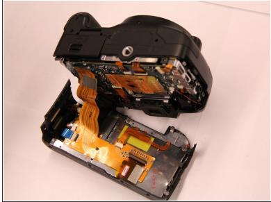
Using the spudger and plastic opening tool, pry the back of the camera loose.
