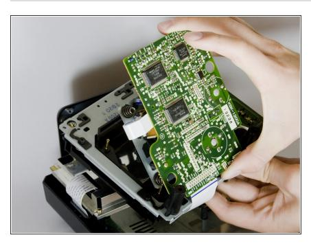
Carefully remove the CD tray from circuit board.
