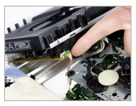
Carefully unplug the wire connected to optical reader.
