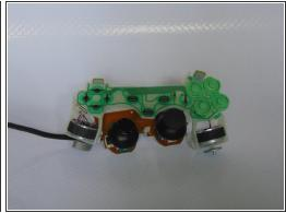
Using a pry tool separate the two controller pieces
