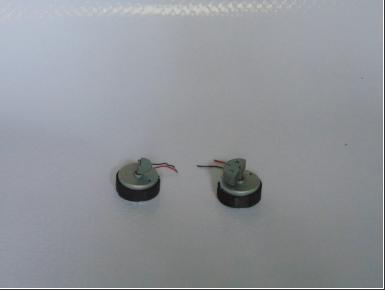
When I lifted the controller out of the chassis one of the dual shock motors fell off it soldering. I removed the other one.
