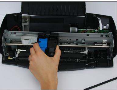
Slide the ink cartridge from the right side to the middle left so it is out of the way.
