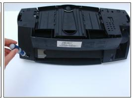
Use a Phillips head #2 screwdriver to remove the 4 screws located on the bottom of the Dell Photo Printer 720.
