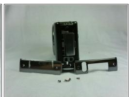
Remove the side panels by unscrewing the Phillips head screws on both sides of the camera.
