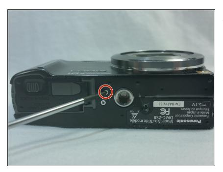
Turn the camera over so that the bottom is facing you. Using a Phillips head screwdriver, unscrew the small screw located on the bottom of the camera.
