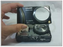
Carefully lift the front panel away from the camera until it is completely separated.
