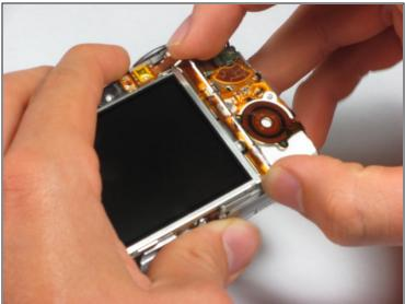
• Remove the two metal frames that hold the LCD panel in place.
