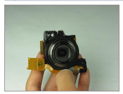
• Gently remove the camera lens from the rest of the camera.
