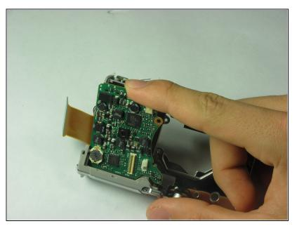
Now the motherboard can be gently removed from the metal casing.
