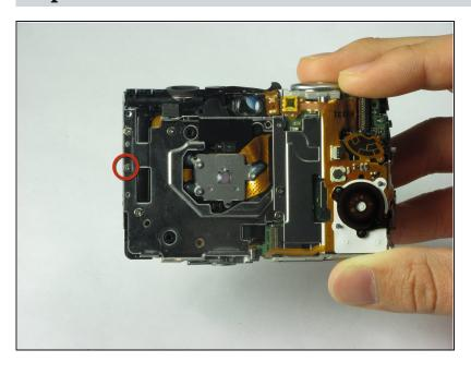
Remove the 1.85 mm #00 Phillips located on the left side of the camera.
