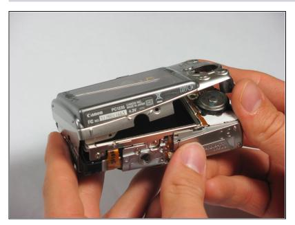
Slide the back casing (with the screen protector) off to reveal the LCD and back wiring.
