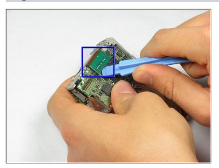
Use a spudger or a flathead screwdriver to release the motherboard cable.
