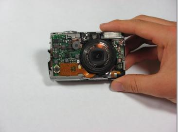
• Gently pull the front cover straight out from the camera. This will expose the wiring on the front of the camera.
