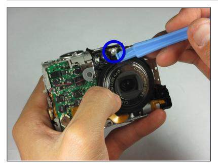
Use a spudger or a flathead screwdriver and carefully pry out the bulb located in the front of the camera on top of the camera lens.
