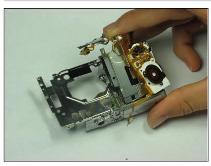
The whole ribbon and metal casing can now be easily removed from the remains of the camera.
