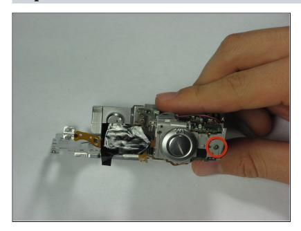
Remove the 2.6 mm Phillips #00 located near the shutter release button.
