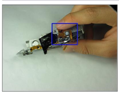
Use a prying device or your fingers to release the ribbon from their respective holders located at the top of the camera.
