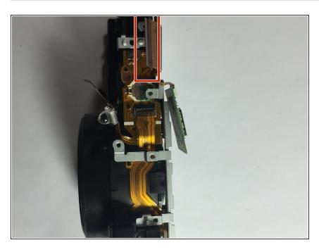
Remove the tabs which will slide out with a chip. The chip is attached to the GPS.
