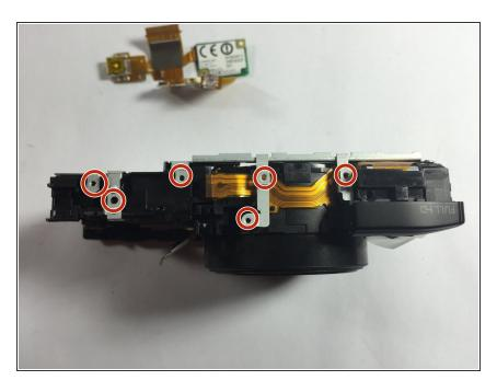
Remove the screws on top of the camera.
