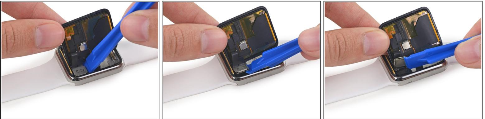
**i** The display and digitizer cable connectors are secured beneath a small metal bracket that is adhered to the speaker.
