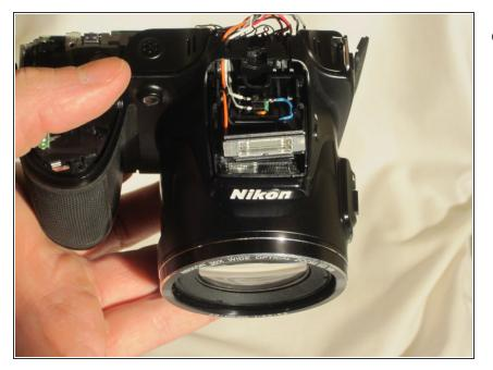
Once the panel has been removed, the bulb is accessible and can be replaced.
