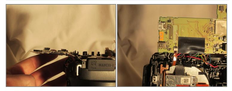
• Once the flex circuits are removed, the motherboard can be lifted and the device can be accessed for replacement.
