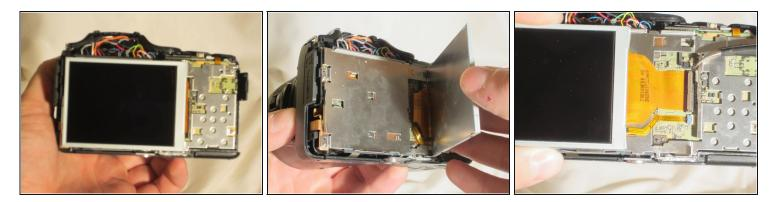
• Remove the front casing to expose the LCD screen and wires.
