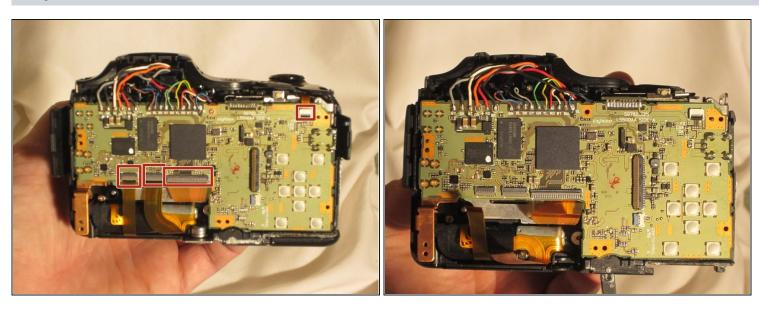
• Using the pointed end of the spudger, lift the hinges that secure these four flex circuits.
