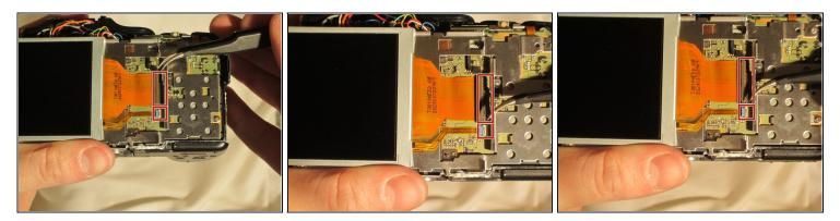
• Using the tweezers, lift the hinges connecting the two ribbon wires to the camera.
