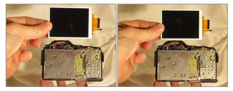
• Once the flexible ribbon wires are disconnected, remove the LCD screen.
