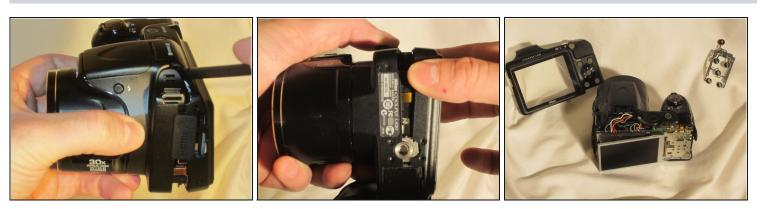
• Using the spudger, move around the casing, carefully separating the rear housing from the camera assembly.
