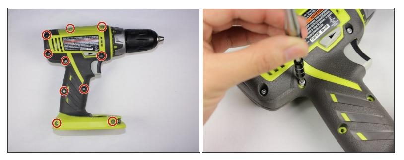
Use a Torx T10 screw driver to unscrew all ten 13.5 mm screws from the drill casing to gain access to the interior.
