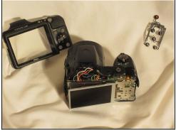
Using the spudger, move around the casing, carefully separating the rear housing from the camera assembly.
