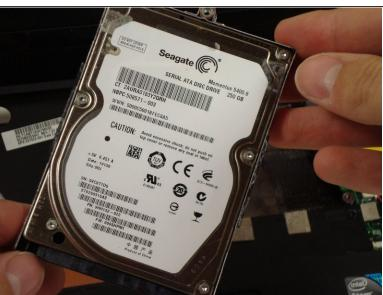
Pull up on the tab to remove the hard drive.
