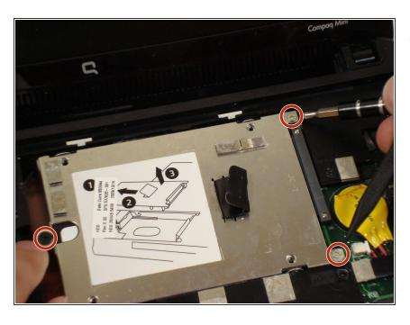
Remove the three screws holding the panel in place.
