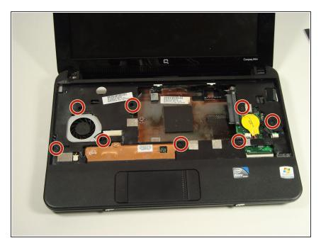
Remove the eight screws that are from the plastic top cover.
