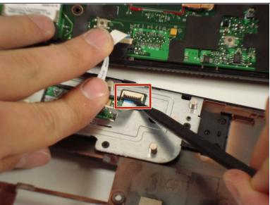
Remove the cable by carefully pulling it up.
