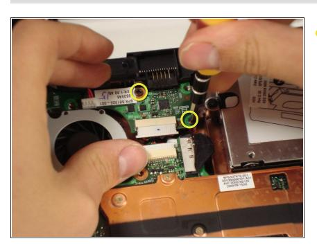
Remove the two screws keeping the board in place.
