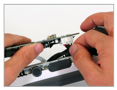
• Disconnect the two white connectors from the bottom of the motherboard.
