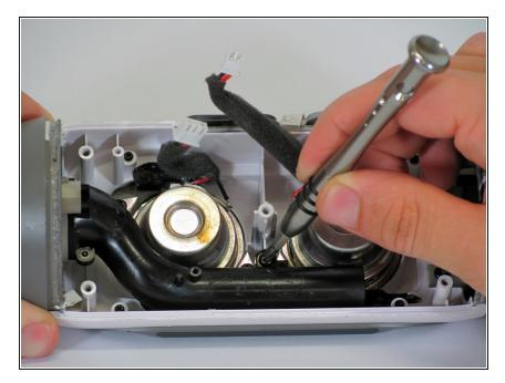
Using the PH1 screwdriver, remove the 9mm Phillips screw that connects the black tube to the device's interior.
