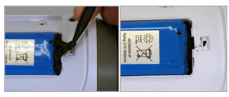
Use a spudger to carefully remove the liquid electrical tape that holds the battery inside the battery compartment.
