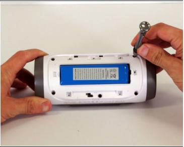
Remove the four 16 mm screws from the white plastic casing using the PH2 screwdriver.
