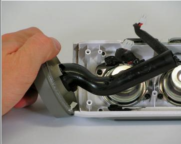
Slowly but firmly pull the grey cap off the device. This will provide complete access to the speakers.
