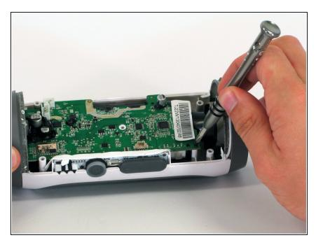
• Remove the 9 mm Phillips screw in the corner of the motherboard.
