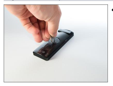
• Using a quarter, turn the battery cover 1/8th of a turn counterclockwise.
