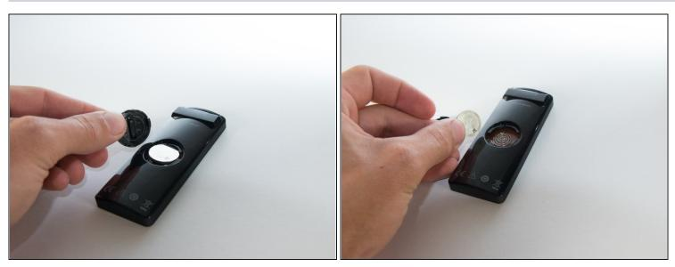
• Remove cover and battery. The new battery should be placed with the positive (flat) side facing up.
