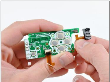
• Use your fingernail or the edge of a plastic opening tool to flip up the retaining flap on LED indicator ZIF connector.
