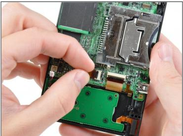
Use your fingernail or the edge of a plastic opening tool to flip up the retaining flap on power board ZIF connector.
