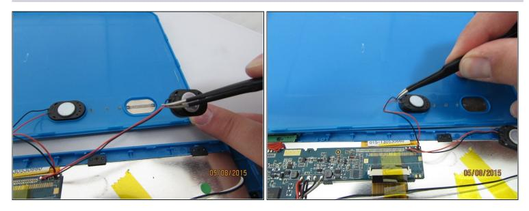
• Gently remove the speakers from the back case with <u>tweezers</u> and set the case aside.
