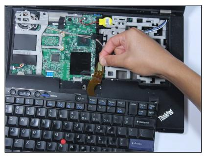
Remove the orange cable by lifting up on the tab on the end of the ribbon connection.
