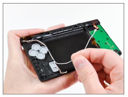
De-route the Wi-Fi antenna cable from its slot in the bottom front bezel.
