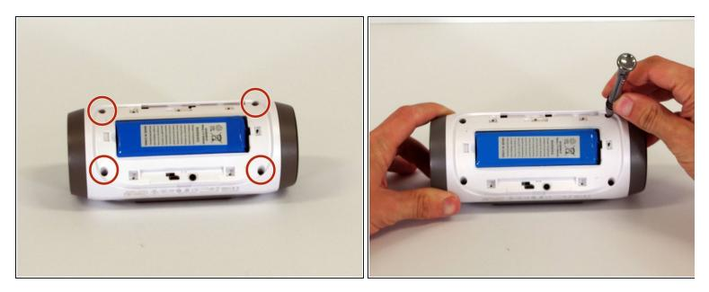
• Remove the four 16 mm screws from the white plastic casing using the PH2 screwdriver.
