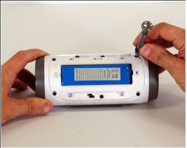
Remove the four 16 mm screws from the white plastic casing using the PH2 screwdriver.
