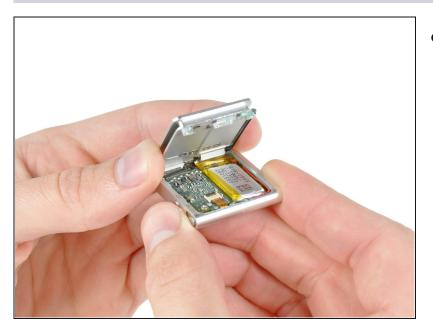
• Remove the rear panel from the Shuffle.
