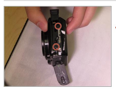
After removing the panel, remove the two black M1.4 X 3.5 Phillips head screws.
