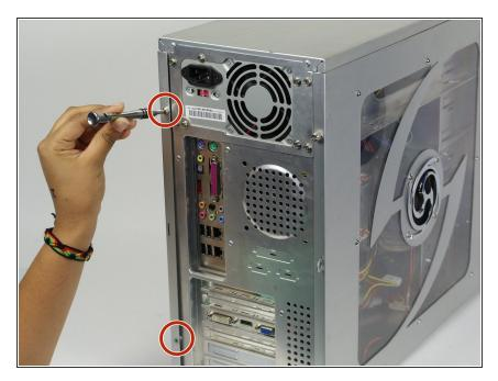
Remove two Phillips #2 head 5mm screws from the back side of the computer case.
