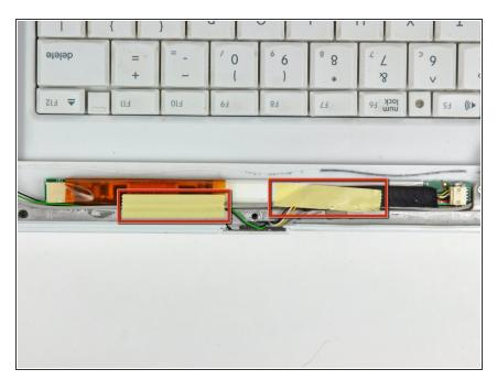
Remove the two pieces of yellow tape covering the inverter/AirPort cables.
