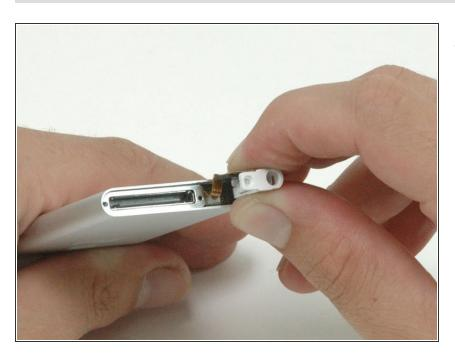
Slide the headphone jack out until the white plastic housing is no longer held in place by the metal casing.
