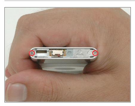
Remove the two Phillips #00 screws from the top of the iPod.
