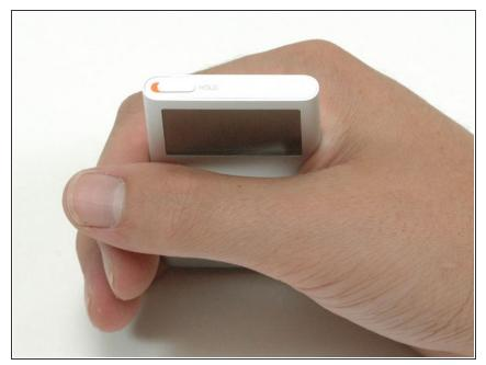
Before opening your iPod, ensure that the hold switch is in the locked position.
