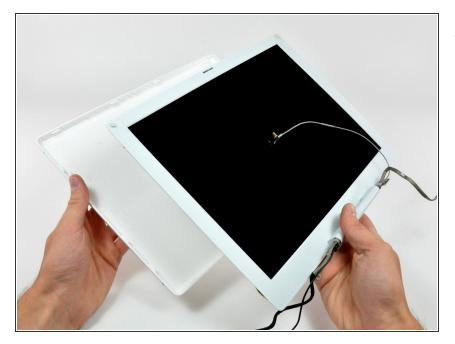
• Lift the rear bezel off the display.
