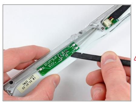
Use the flat end of a spudger to remove the antenna board from the front bezel.
