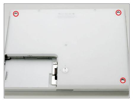
• Remove the three newly-revealed Phillips screws.
