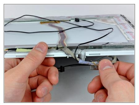
• Remove the display data cable from the display.
