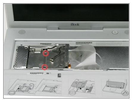
• Remove the two Phillips screws that secure the RAM shield.
