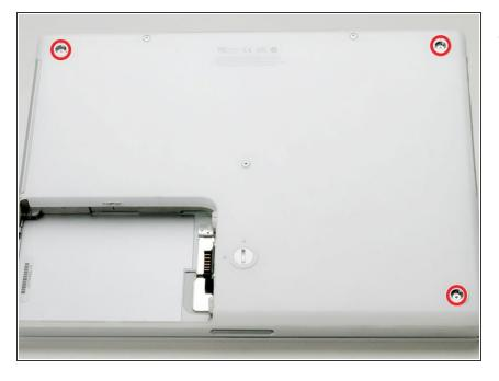
Remove the three newly-revealed Phillips screws.
