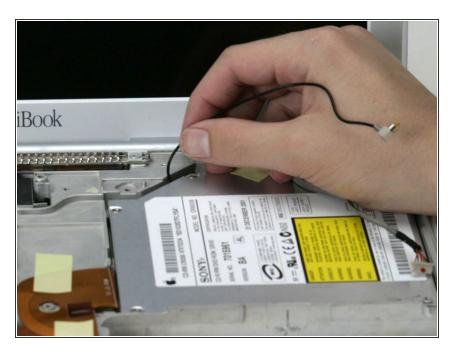
Deroute the AirPort antenna cable from beneath the optical drive.
