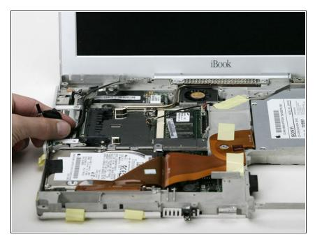
Deroute the display data and microphone cables, removing tape as necessary.
