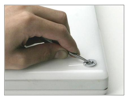
Use a spudger or small flathead screwdriver to pry up the three metal rings that housed the rubber bumpers.
