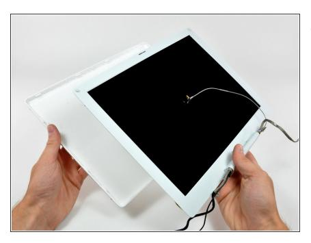
Lift the rear bezel off the display.
