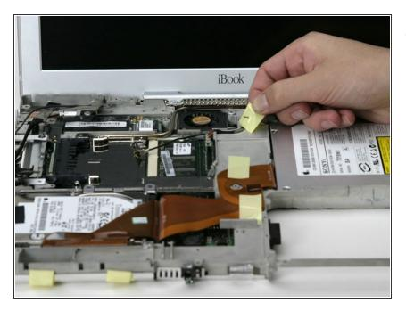
Peel back the yellow tape securing the inverter cable to the metal framework.
