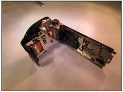
• Pull the plastic cover on the back out and up slightly until the back feels like it's free, then pull back on the plastic (The top cover piece and back will be detached).
