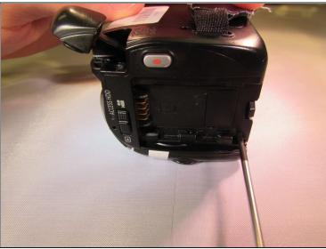
• Remove the black 4 mm screw from the back of the camcorder underneath where the battery would have been.
