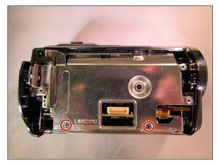
Unscrew the two black 4 mm screws from metal casing around the motherboard.
