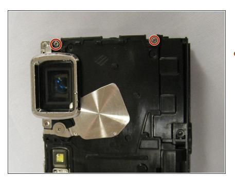
Using a Phillips 00 screwdriver, unscrew the 9mm screws on the top of the camera to the right of the flash.
