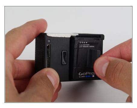
Pull the battery out using the tab.
