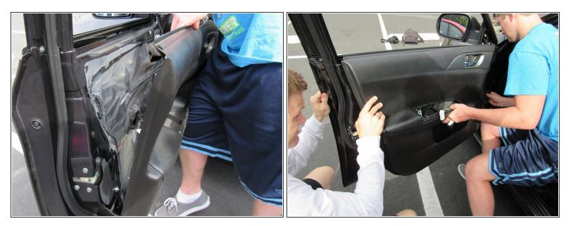
Finish pulling the door off of the frame, now that all the clips have been disconnected.
