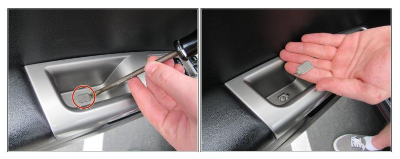
• Pry up the plastic tab from inside the handle located on the front door armrest.
