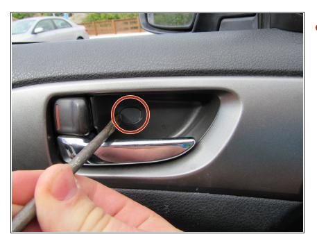
Pry up the plastic tab from inside the door handle housing.
