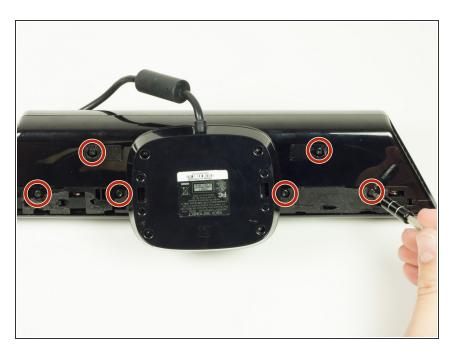
Unscrew the six 12mm T10 Torx screws.
