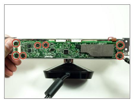
Unscrew the seven 6.5mm T10 Torx screws.
