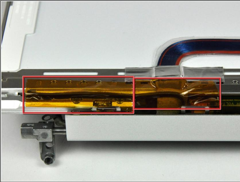
**i** If necessary, remove the two pieces of tape covering the inverter leads.
