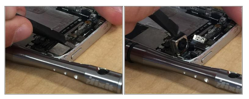
Remove the connector next to the camera from its port and then lift the camera module away from the phone.
