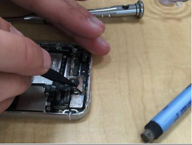
Remove the metal cover near the camera module to reveal the screw and camera connectors
