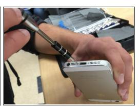
To start the teardown, remove the two screws near the bottom.
