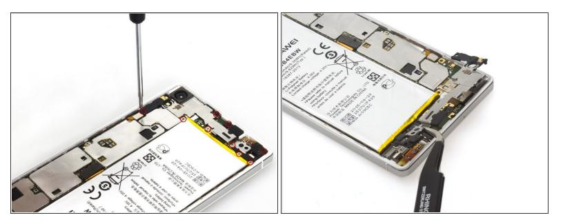
Twist off those nine screws and remove the bracket.
