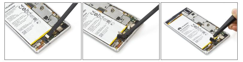
There is adhesive under the vibration motor, so release the connector and pry up to remove the assembly.
