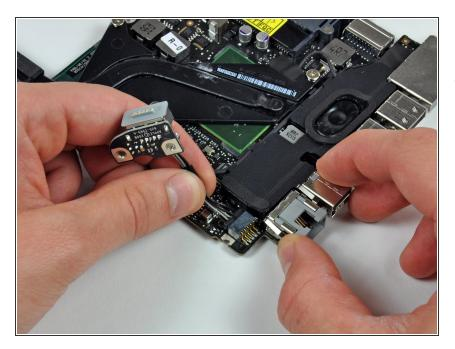
Disconnect the DC-In board by pulling its connector away from the socket on the logic board.
