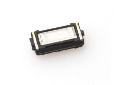
Pry up and remove earpiece speaker finally.
