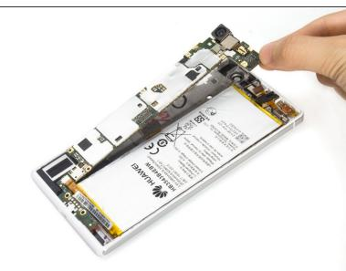
Release all connectors on the board and remove motherboard carefully.
